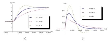
**Figure 2.** Voltage on capacitor a) and current through elements of circuit b) for  $C=2 \mu F$ , L=2mH,  $V_S=12V$ ,  $V_0=5V$ .
