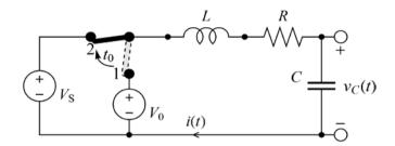
Figure 1. Electrical circuit of second order with serial link of coil, resistor and capacitor.
